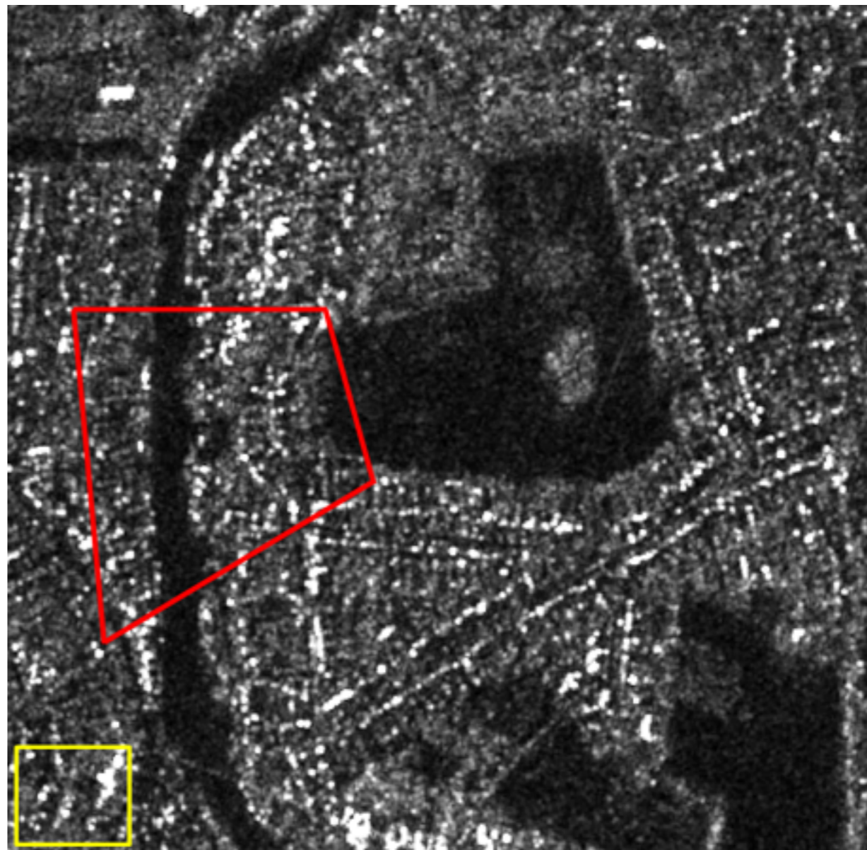
CSK sub-image (1 x1 km) of Thames flood in Wraysbury (dark areas are water). Red outline shows the area covered by the aerial photo.
