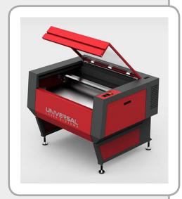
The Laser Cutter has a bed made of Aluminum "Honeycomb" that supports material and allows the extraction of fumes and particles from below. Make sure that the "Honeycomb" surface is clear of all debris.
