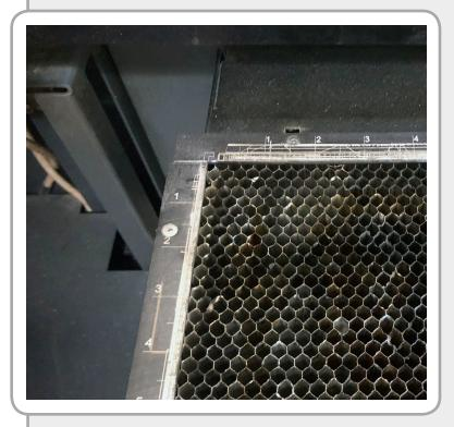
Make sure the table is square to the rulers in the bed of the laser cutter by sliding it back and to the left until it stops.
