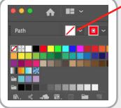
No fill color should be assigned to objects for laser cutting. Set the fill color to None in the control bar. Clicking on the displayed color will open the drop down palette.
