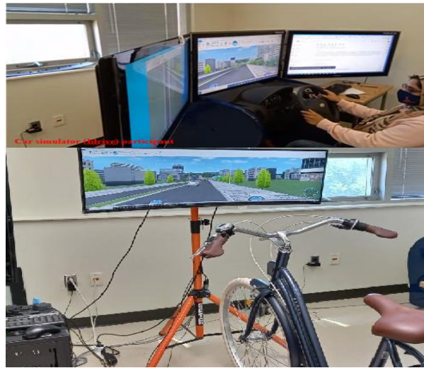
Figure 10 Integration of bike and car simulators
