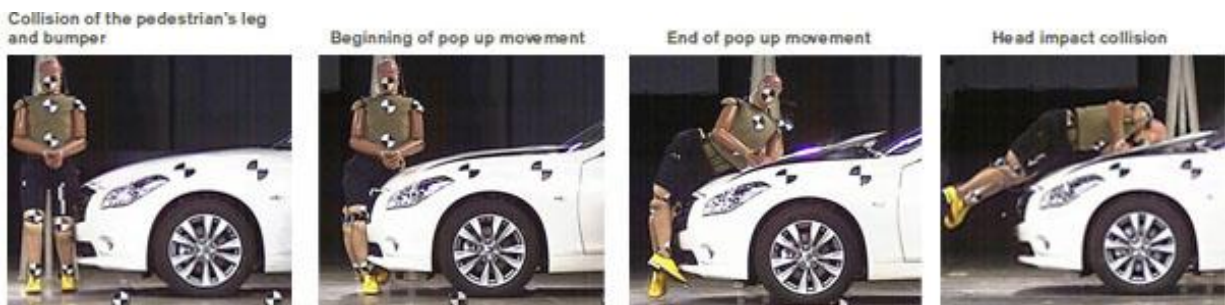
FIGURE 33 Stages of EPP (54)
