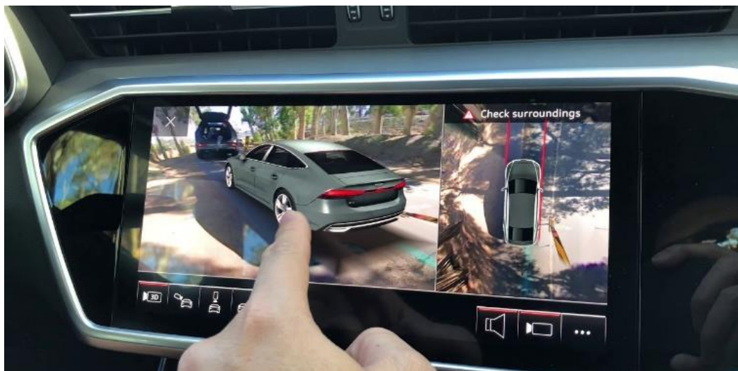
FIGURE 28 Audi 360-degree cameras (45)
