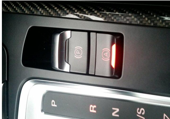
FIGURE 25 Audi Hill Hold Assist (44)
