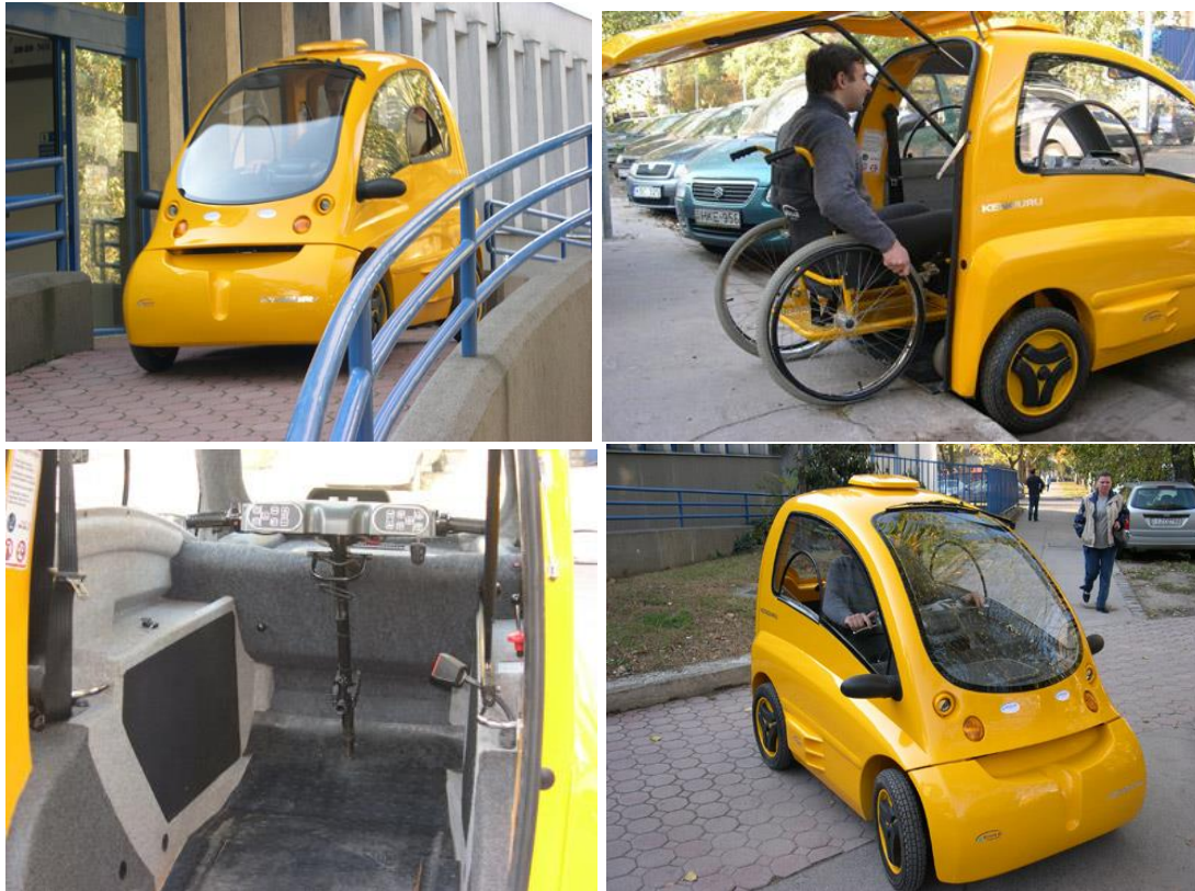
FIGURE 50 Kenguru EV Made for Wheelchair Users
