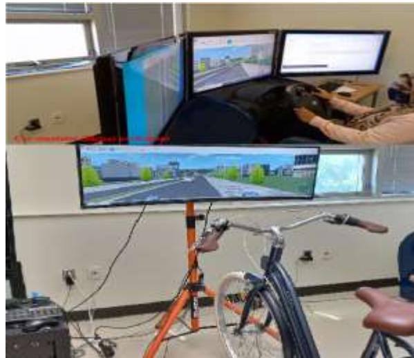
Figure 2 Integration of bike and car simulators
