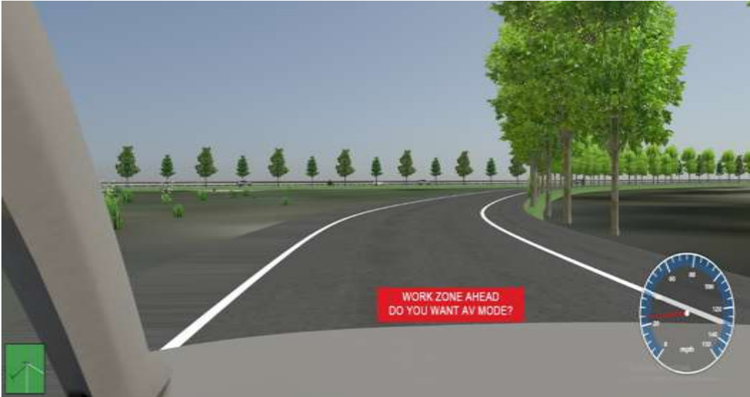
Figure 8: Connected & Automated Vehicle function showing work zone entrance warning.
