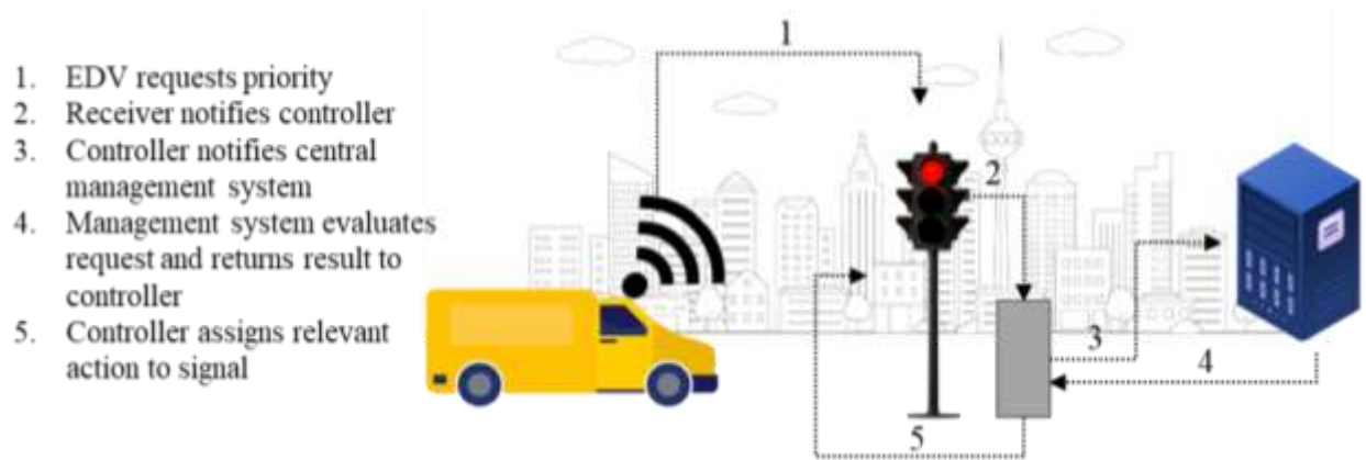
Figure 5 Vehicle-to-infrastructure communication mechanism
