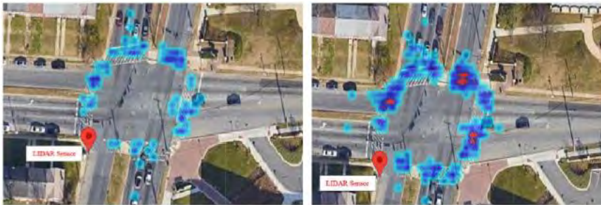
Figure 20 Vehicle-Pedestrian Conflicts Heat Map in July (left figure) and August (right figure)
