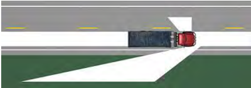
Figure 3: locations of blind spots for a single-unit truck (adopted from (35))
