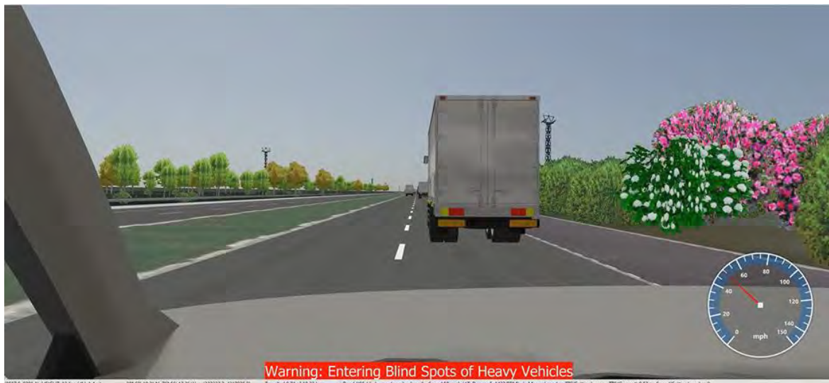
Figure 9: BSW-H triggered in the Area #1 at the Rear of the Truck
